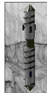
Figure 2. CAD Rendering of the Inchworm Deep Drilling System concept. Uses a two part inchworm motion to thrust into ice.
